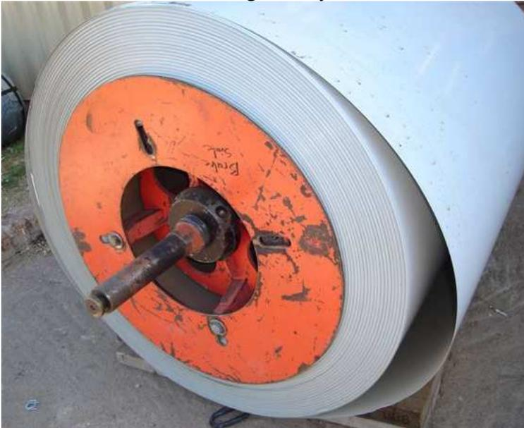
This chromadeck steel is glued with a 2ply (PU) polyurethane glue on the EPS. When the EPS is boxed on both sides of the EPS with chromadeck it makes it strong and durable
