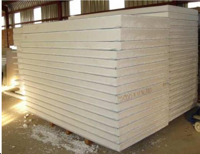
Panel manufacturers use different types of insulation mainly EPS, PU and rock wool. We use only EPS insulation due to its strong structural strength. All EPS panels that are manufacture by Africhill is fire retardant. Generally EPS panels are made with a lot of hand labour, but with our (and some competitors) continues sandwich panel machine it is mostly automatic, computerized and mechanically driven.
